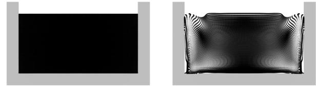
**Figure 7:** *Simulation of a stationary pool with (left) and without (right) density correction. Without correction the faces near collision objects appear lighter which causes them to rise under gravity.*
