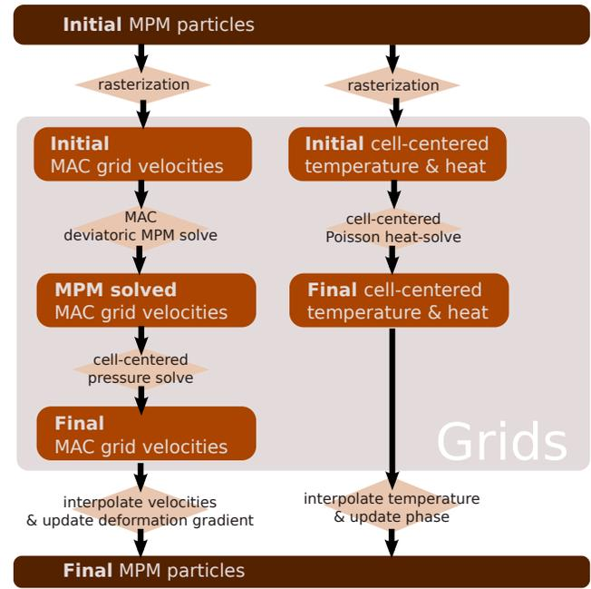
**Figure 4:** Our method benefits from the interplay of grids and particles. In parallel with our mechanical evolution we have a thermodynamic evolution that also uses grids as a scratchpad.
