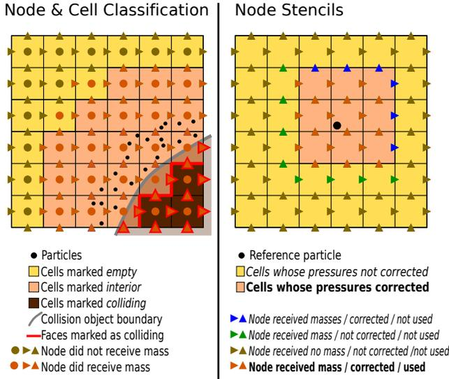
**Figure 6:** *Left figure* illustrates cell classification criteria. Note that faces marked “colliding” are Neumann faces for the Poisson solve and yellow cells marked “colliding” are Dirichlet cells for the Poisson solve. *Right figure* shows stencils for a single reference particle. The particle contributes to the green, blue, and orange faces, the pressure solve only corrects orange and blue faces, but our quadratic interpolation touches only the orange faces.
