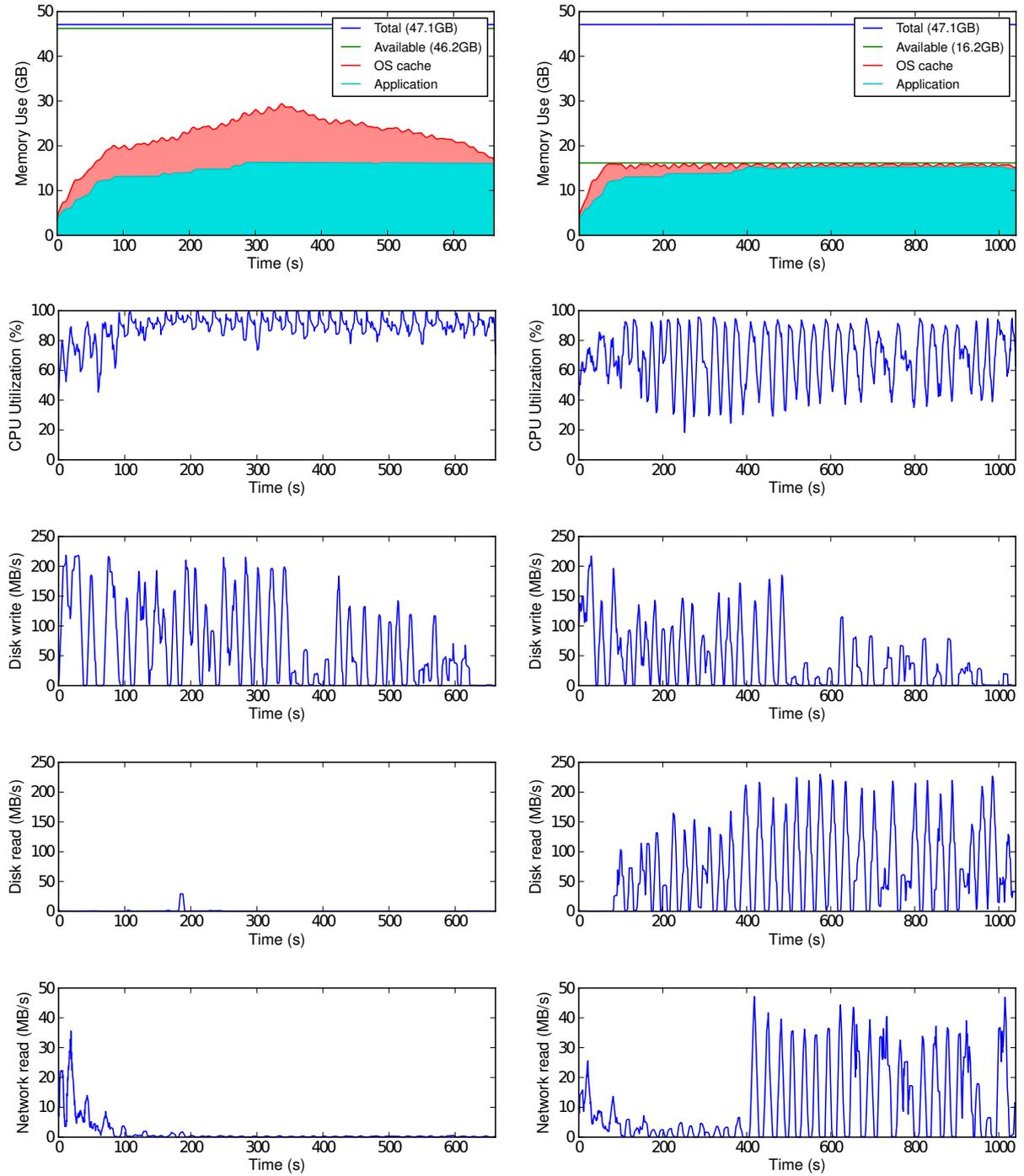
**Figure 10:** System profile during rendering of the interior scene with 4 textures. Left column: with 46.2 GB of available memory, ray batches and textures are cached by the OS, and minimal disk/network reads are required. Right column: restricting available memory to 16.2 GB prevents OS caching, requiring local reads for ray batches and network reads for texture data. Spikes correspond to ray batches being processed.
